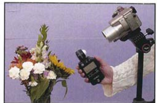
USING AN INCIDENT-LIGHT METER
